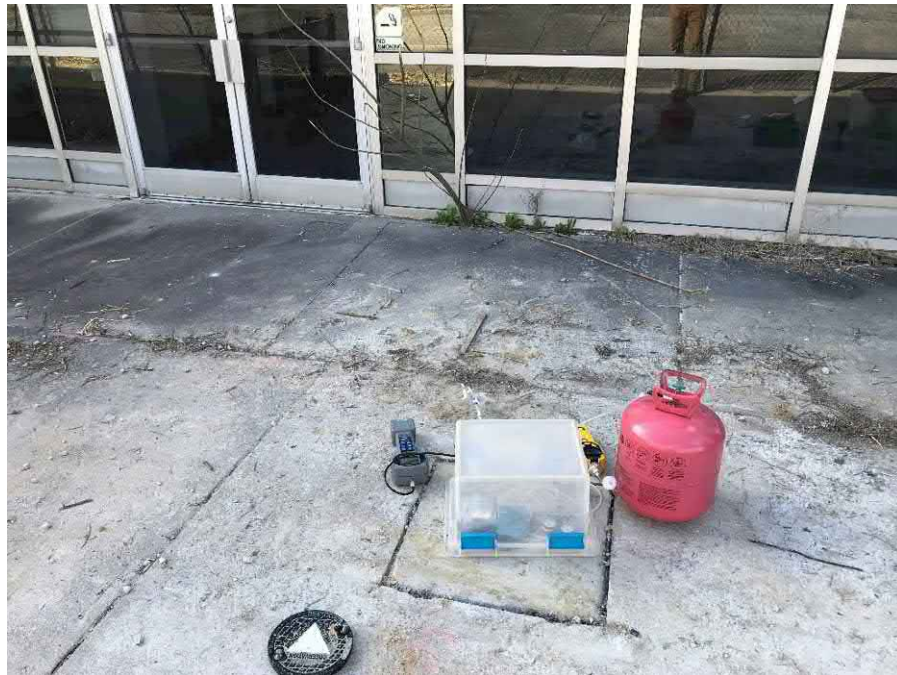
Photo 3 View of SV-15 and helium tracer test set up; facing west.
