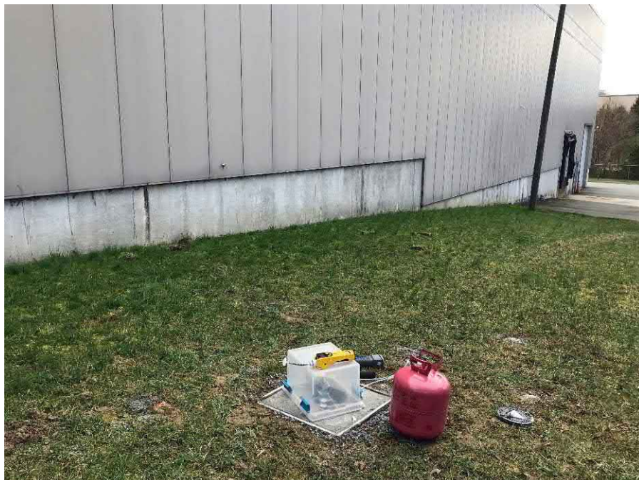
Photo 2 View of SV-14 and helium tracer test set up; facing southwest.
