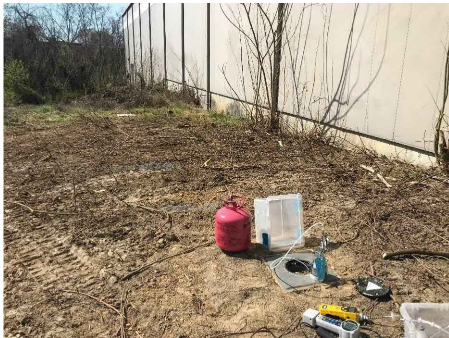
Photo 4 View of SV-16 sample collection following helium tracer test; facing west.
